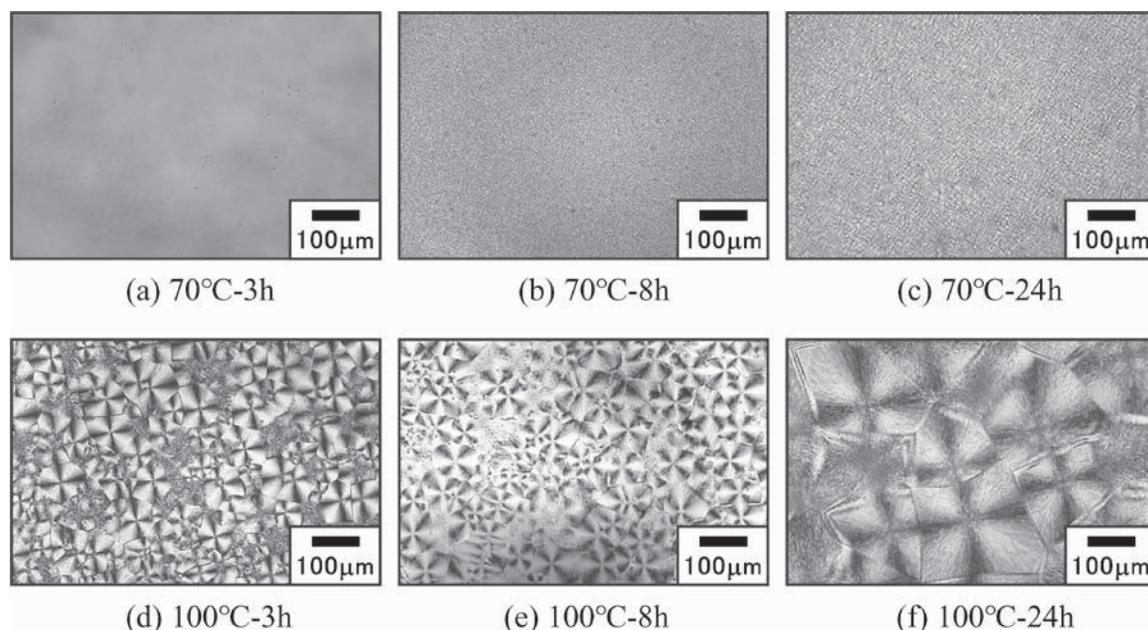
Figure 1 Polarizing microphotographs of microstructures of PLA. (a) 70°C-3hr; (b) 70°C-8 hr; (c) 70°C-24 hr; (d) 100°C-3 hr; (e) 100°C-8 hr; (f) 100°C-24 hr.
