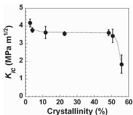
Figure 2 Effects of the crystallinity on fracture toughness of PLA.
